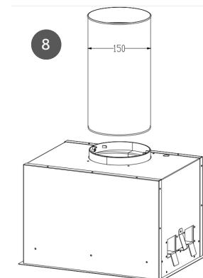
EN 5.10 Installation of the air adapter (reduction)
