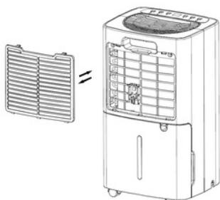
2. Place the T-CLEAN filter in the Filter Frame for proper mounting.
