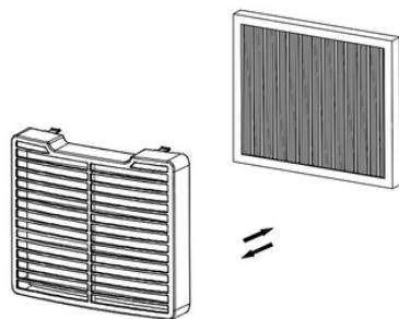
3. Mount the T-CLEAN filter with the frame on the unit
